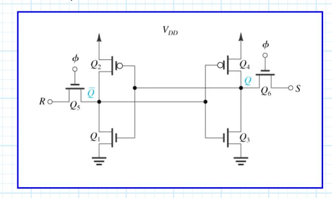
Essentially, when S (Set) is high, the latch is set such that Q is high. Likewise, when R (Reset) is high, the latch is set such that Q is low.
